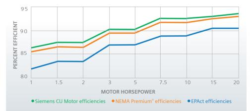
Siemens GP100A motors from 1 to 20 horsepower are available with an optional die cast CU copper rotor that delivers operating efficiencies above NEMA Premium<sup>®</sup> (NEMA MG1, table 12-12) specifications.
