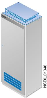
1) Backed with a frame and fine-meshed grille to increase the degree of protection to IP40.
